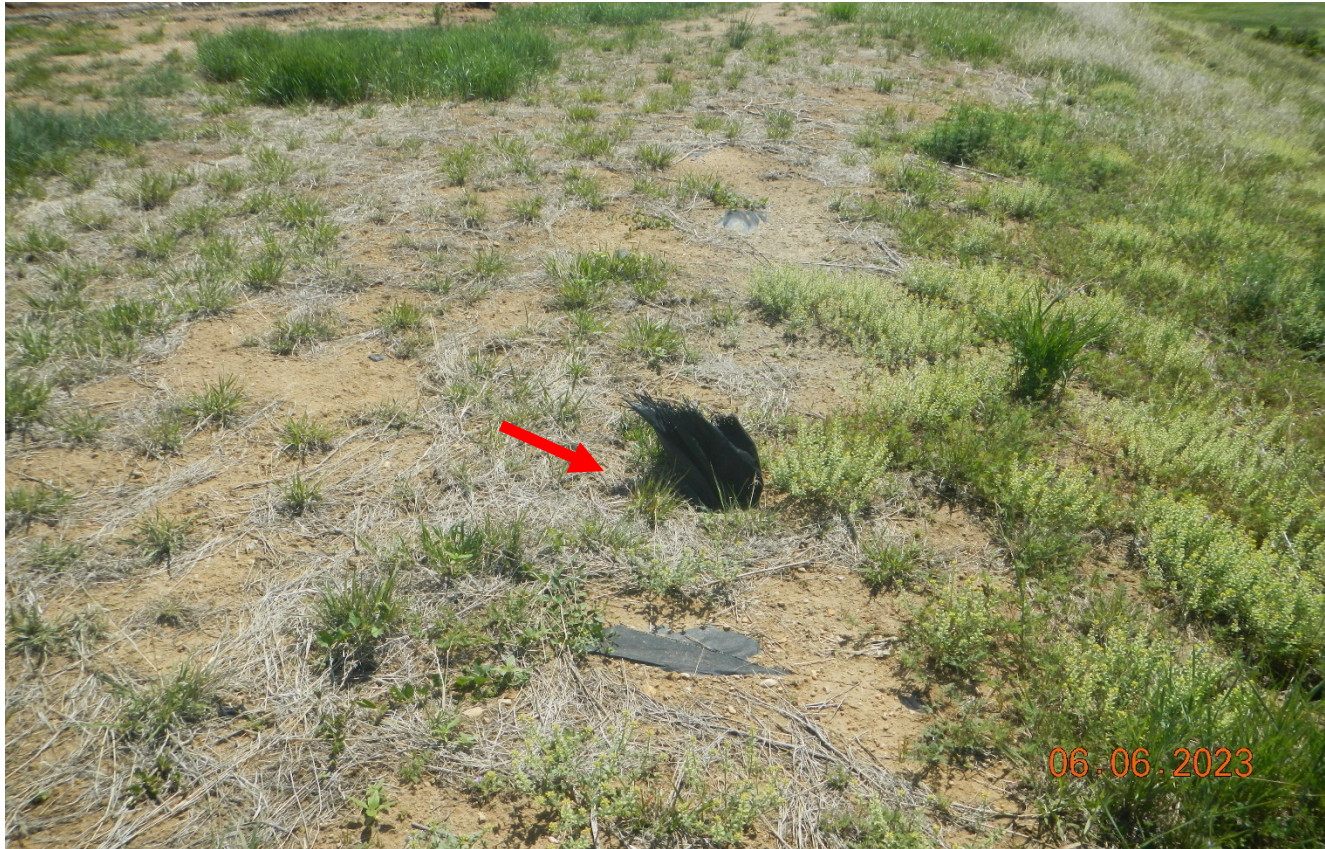
Photo 6. There appears to be liner debris at the surface at the southwest side of the pad.
