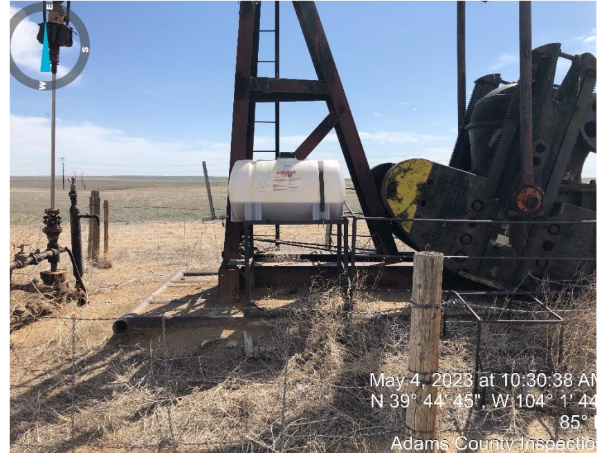
Photo# 6 no secondary containment for chemicals.
