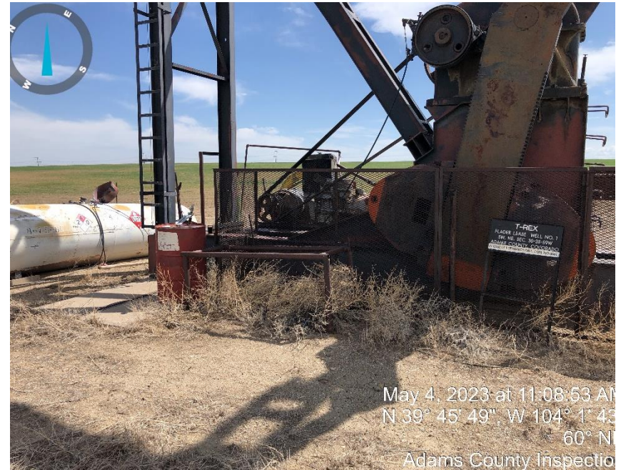
Photo# 8 weeds and no secondary containment for chemical bbl.
