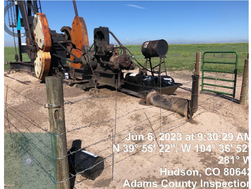
Photo#2 CA:Plastic Buckets around pumpjack. And Secondary containment full
