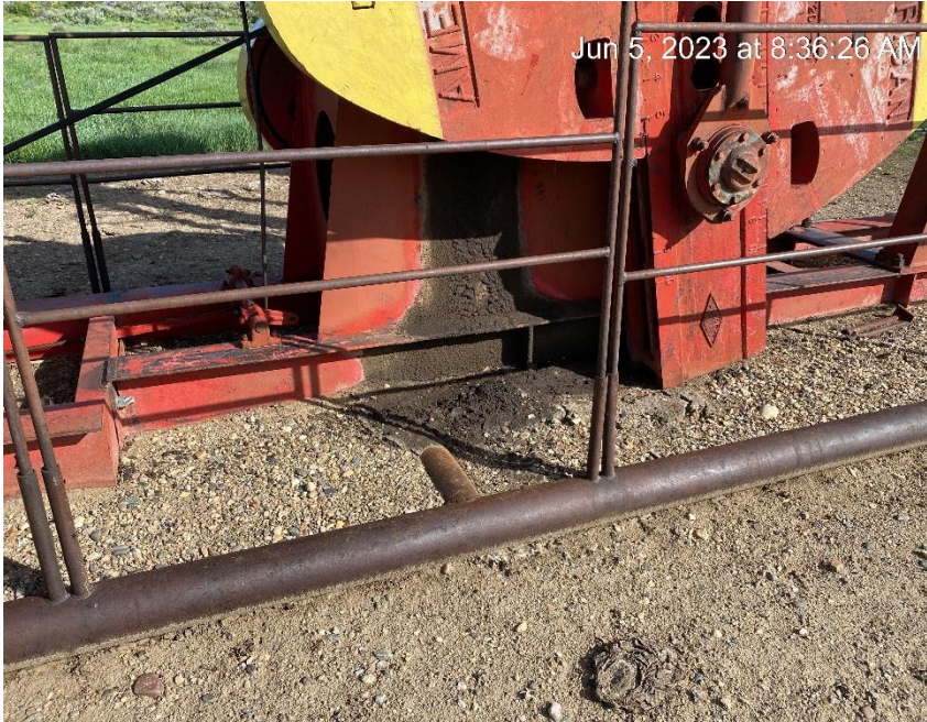
Pumping unit leak with stained soil
