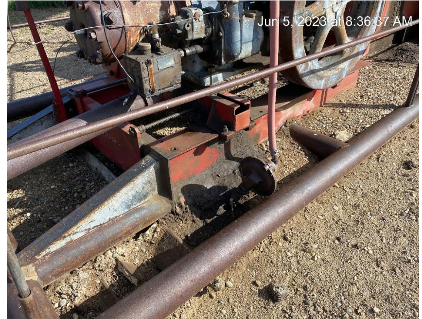
Engine leak(s) with stained soil
