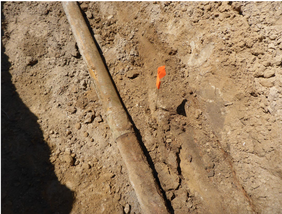
Sample Point G1b (observed stained soil around fiberglass flowline collar)
