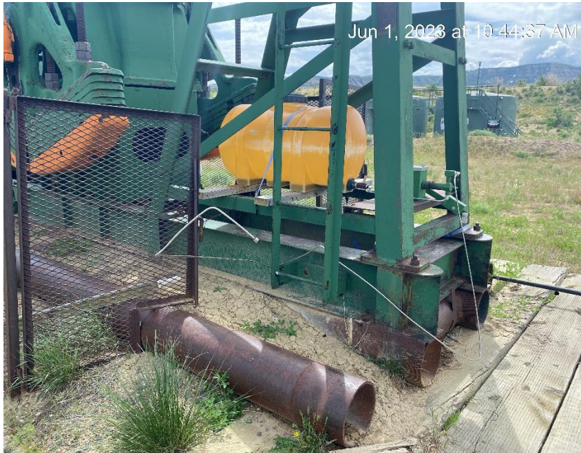
Unlabeled chemical tank. No containment.
