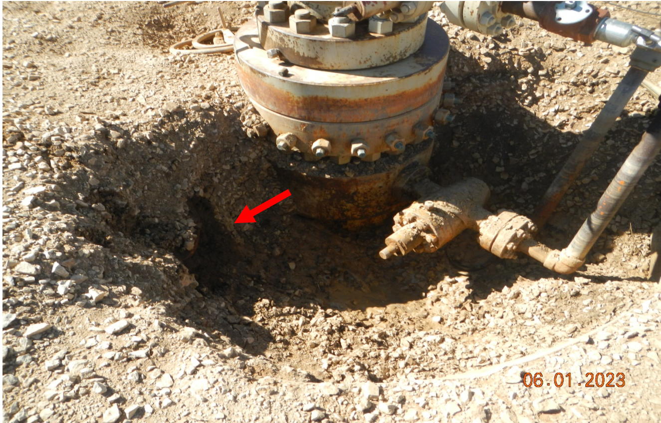
Photo 2. The wellhead is partially excavated and there is oil stained soils at red arrow that needs to be cleaned up.
