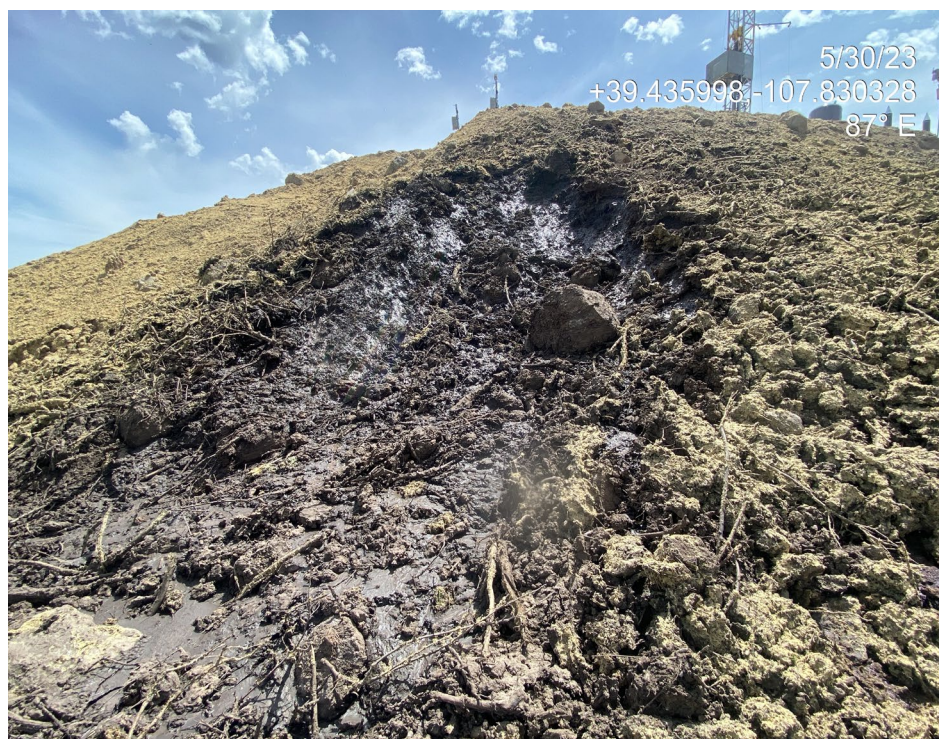
Photo 18. Photos show the top (left) and base (right) of a slump that has occurred in the northwest fill slope of the location.
