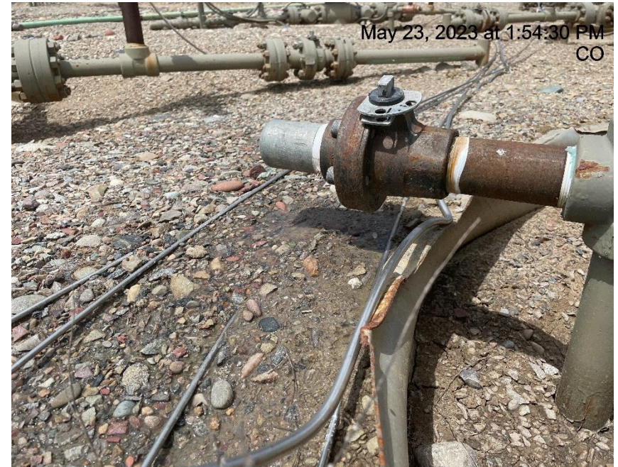
Photo # 8483 Valve on bradenhead leaking fluid onto ground
