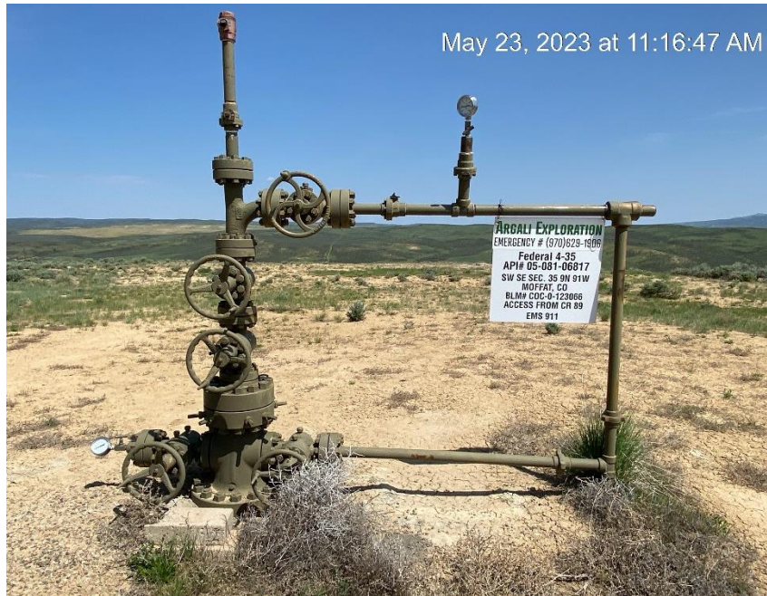
Wellhead and well sign
