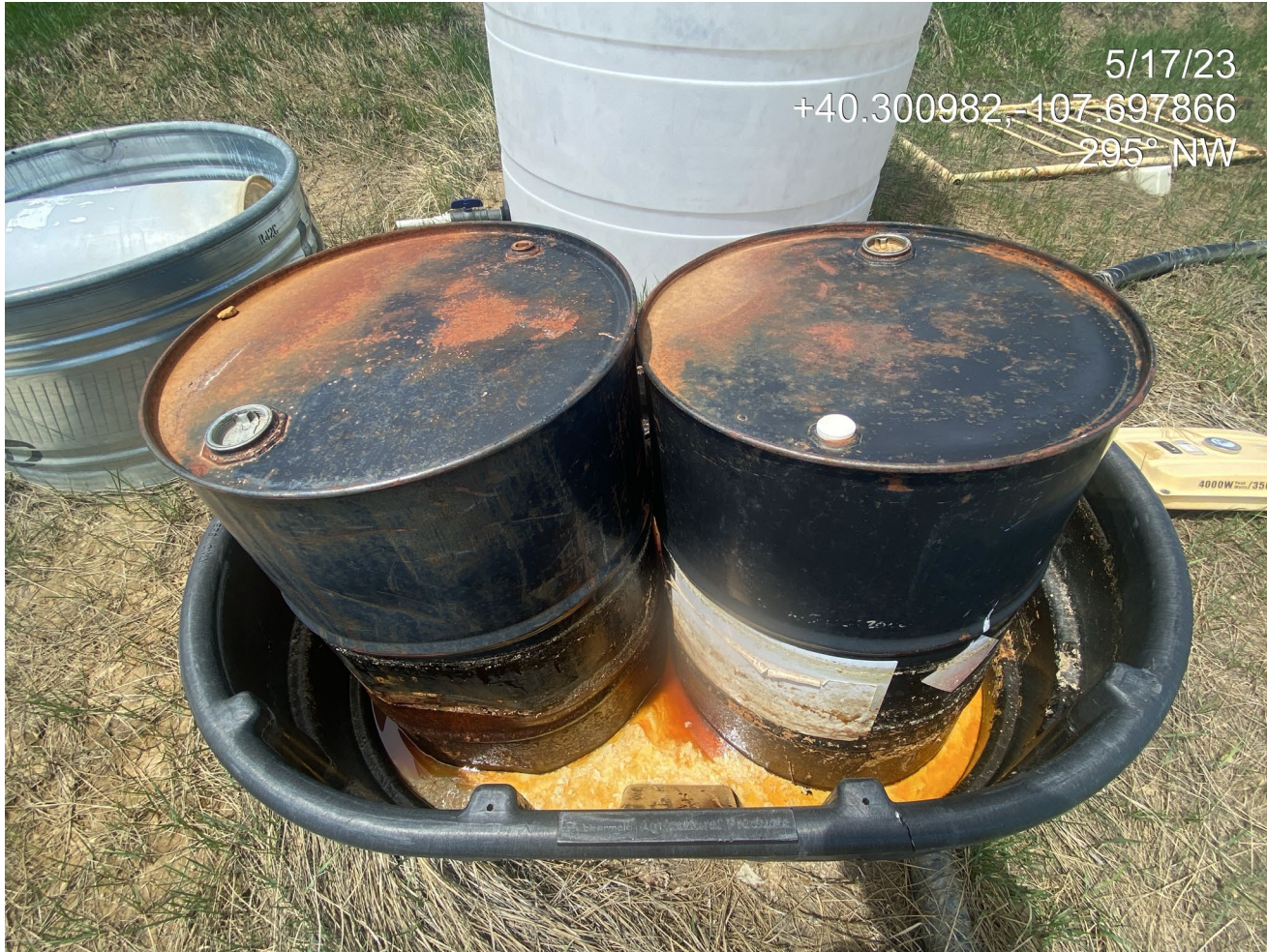
Photo 3. Photo shows storage of leaking chemical drums. No wildlife protection BMPs present to prevent entry into secondary containment.
