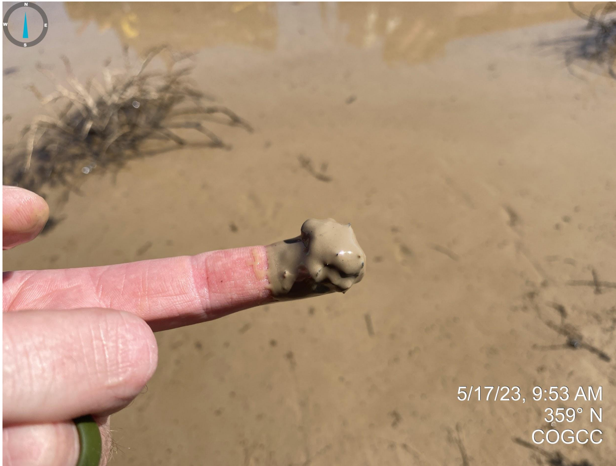
Photo 9. See comments in Photo 6. Unknown fluid did not appear to be the consistency of dirt/soil/stormwater and had noticeable chemical odor and sheen.
