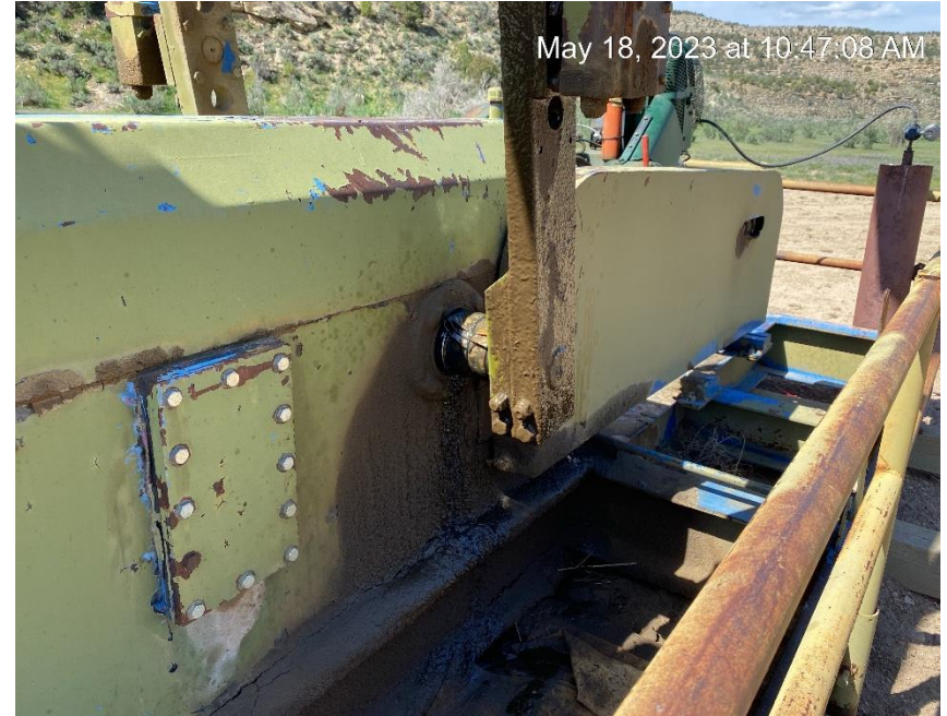
North side gear box leak
