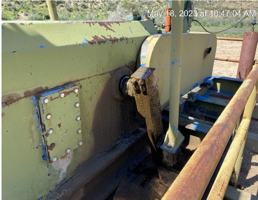
North side gear box leak
