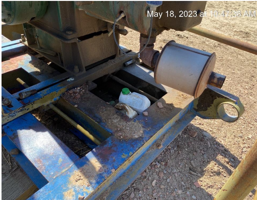
Debris inside skid below engine
