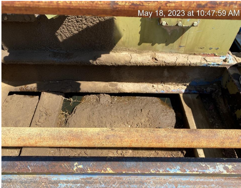
Oil pooling under pumping unit on South side
