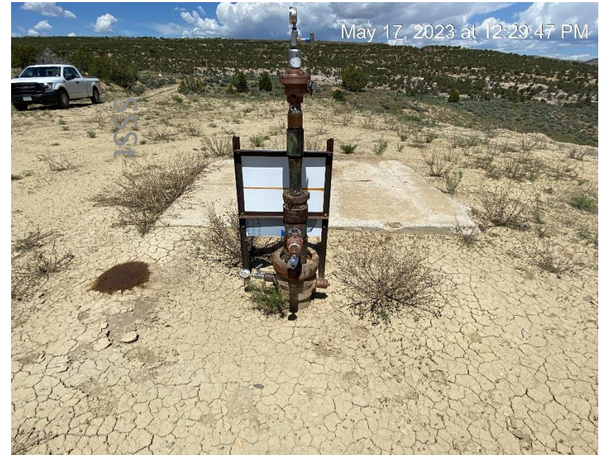
Wellhead. Stained soil.
