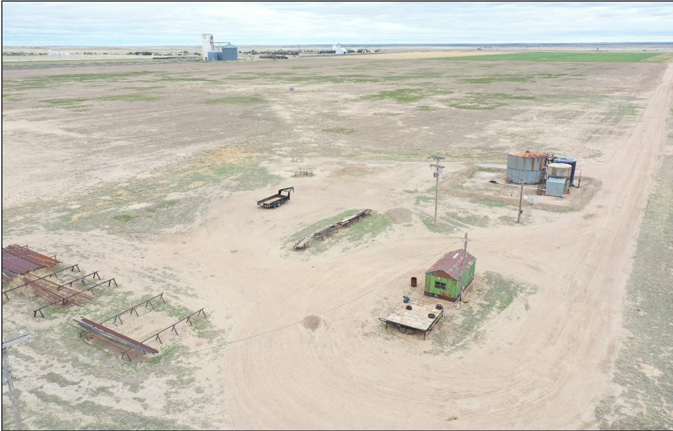
Photo 11. Drone aerial imagery facing southwest toward the tank battery location. The location needs to be reduced in size through interim reclamation to be put back into cropland use. All unused equipment not necessary for use on the location is prohibited and must be removed.
