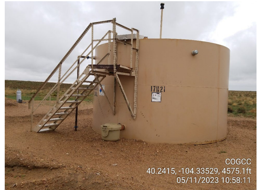
Photo 4 – Tank Battery
