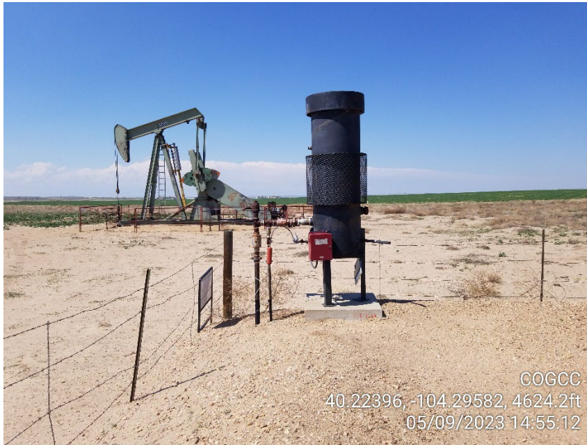
Photo 1 – ECD and Pumping Unit
