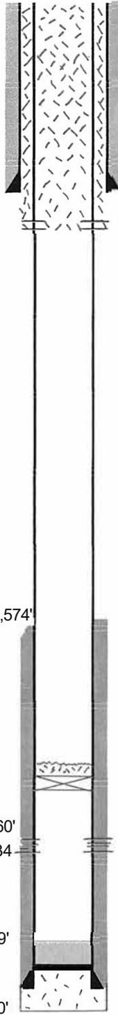
Cement 4.5" casing & 4.5" casing annulus (0 - 456') to surface with 95 sacks class G 15.8 #/gal cement. Yield is 1.15
