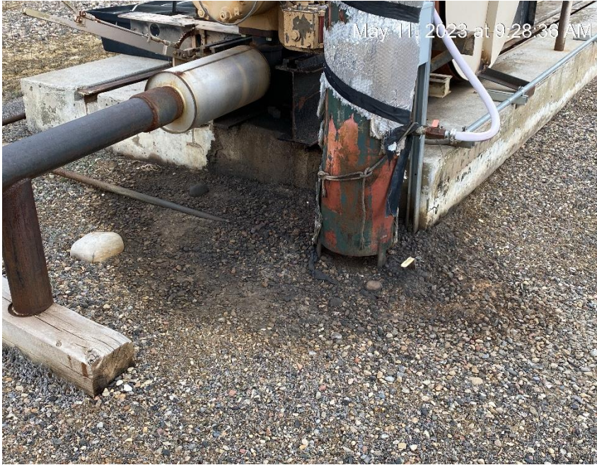
Oily waste from pumping unit engine
