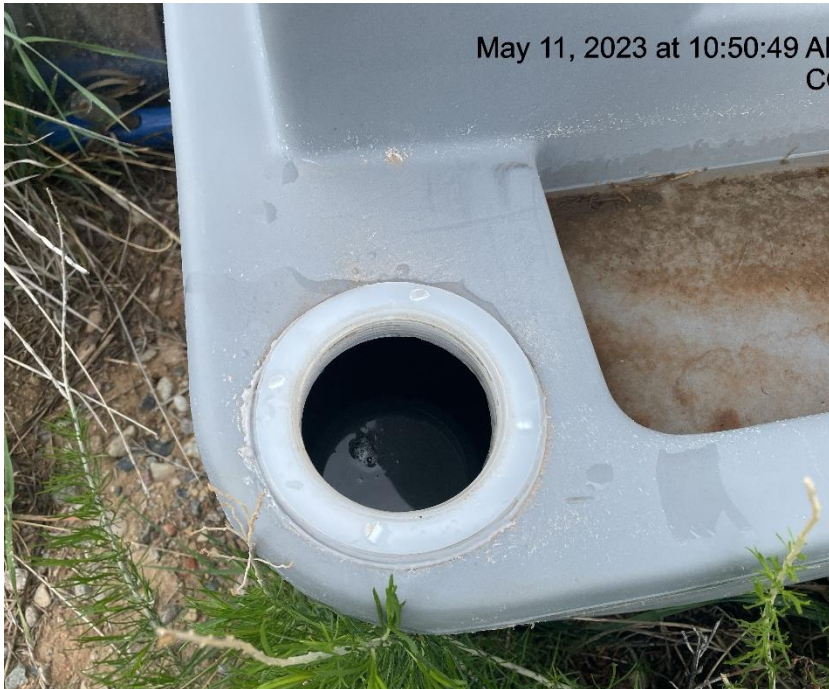
Photo # 7514 Chemical containment full/failure to maintain chemical BMP
