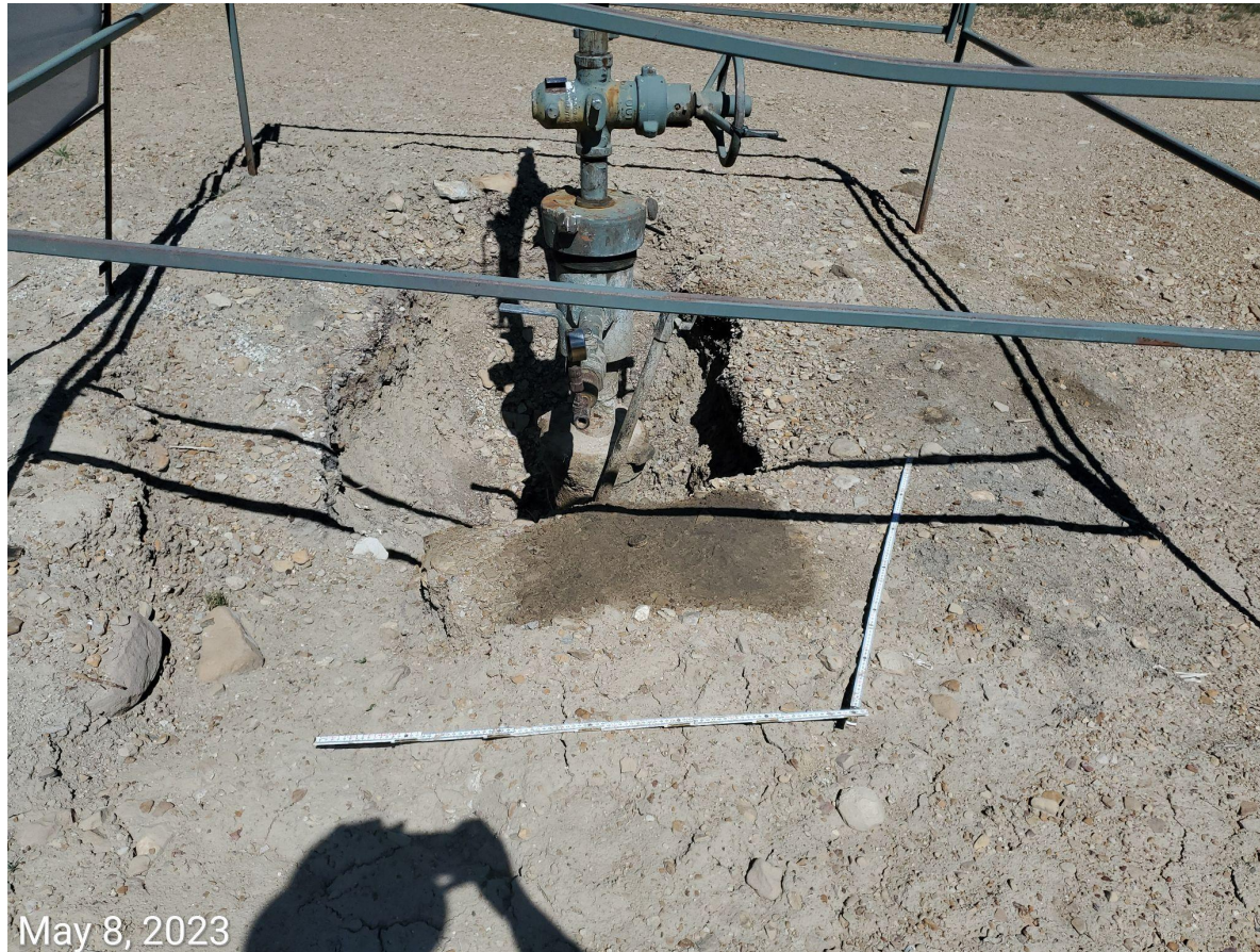
Photo 4: Photo shows stained soils observed at the wellhead. 6 foot measuring stick (3'x3') used for reference.
