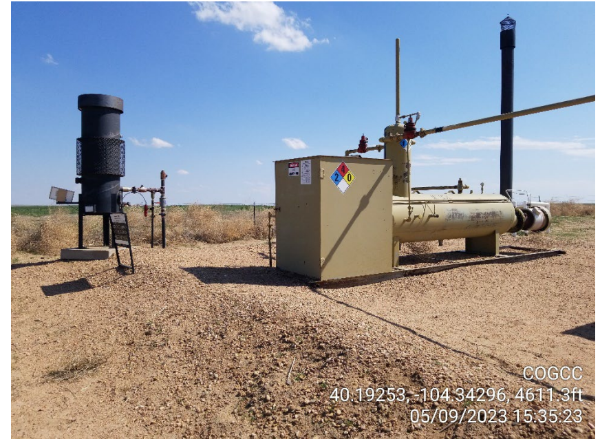
Photo 4 – ECD and Separator
