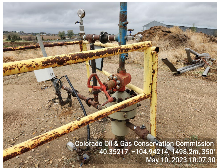
Photo 8: Valve appears to be open
