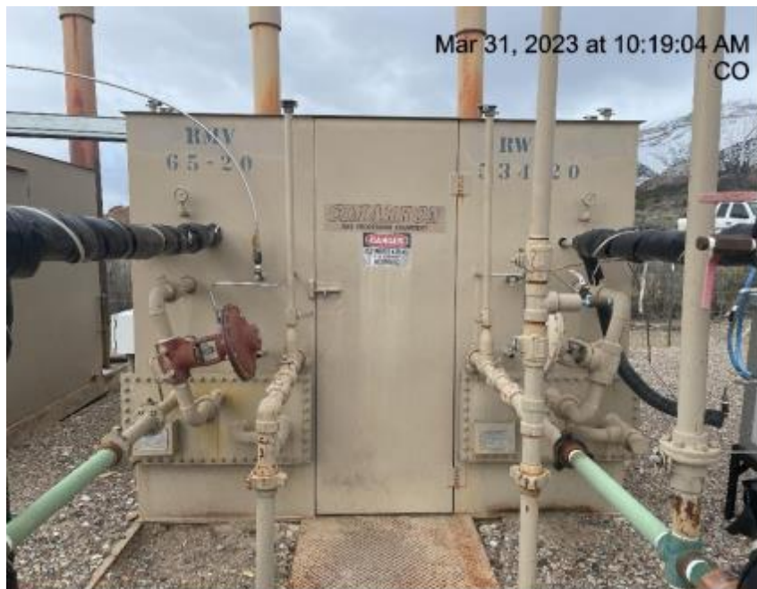
Photo # 3934 From Inspection 708900200 conducted on 03/31/2023 Meter calibration info not conspicuously posted
