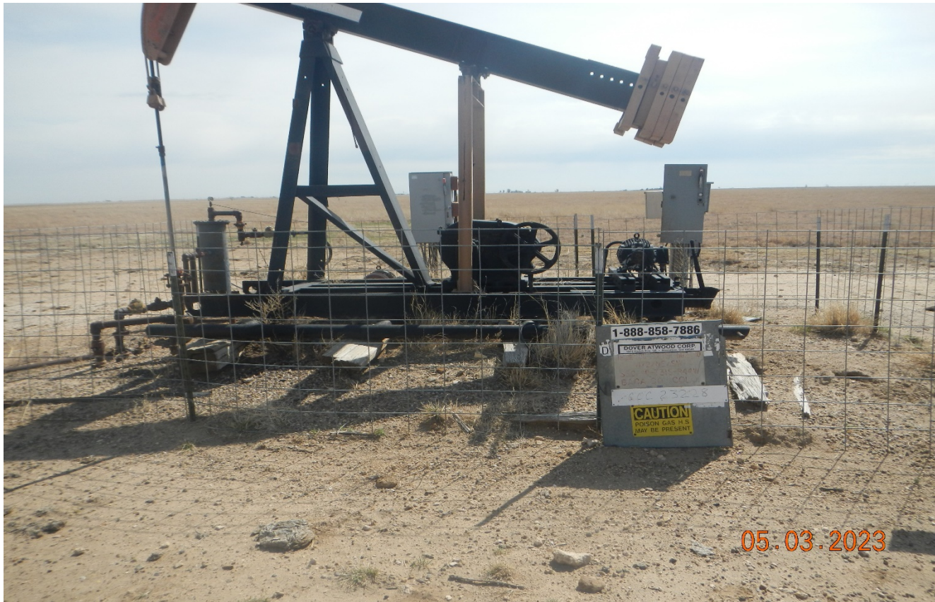
Photo 3. The well sign does not comply with 605. Incorrect Operator Emergency number and missing information.
