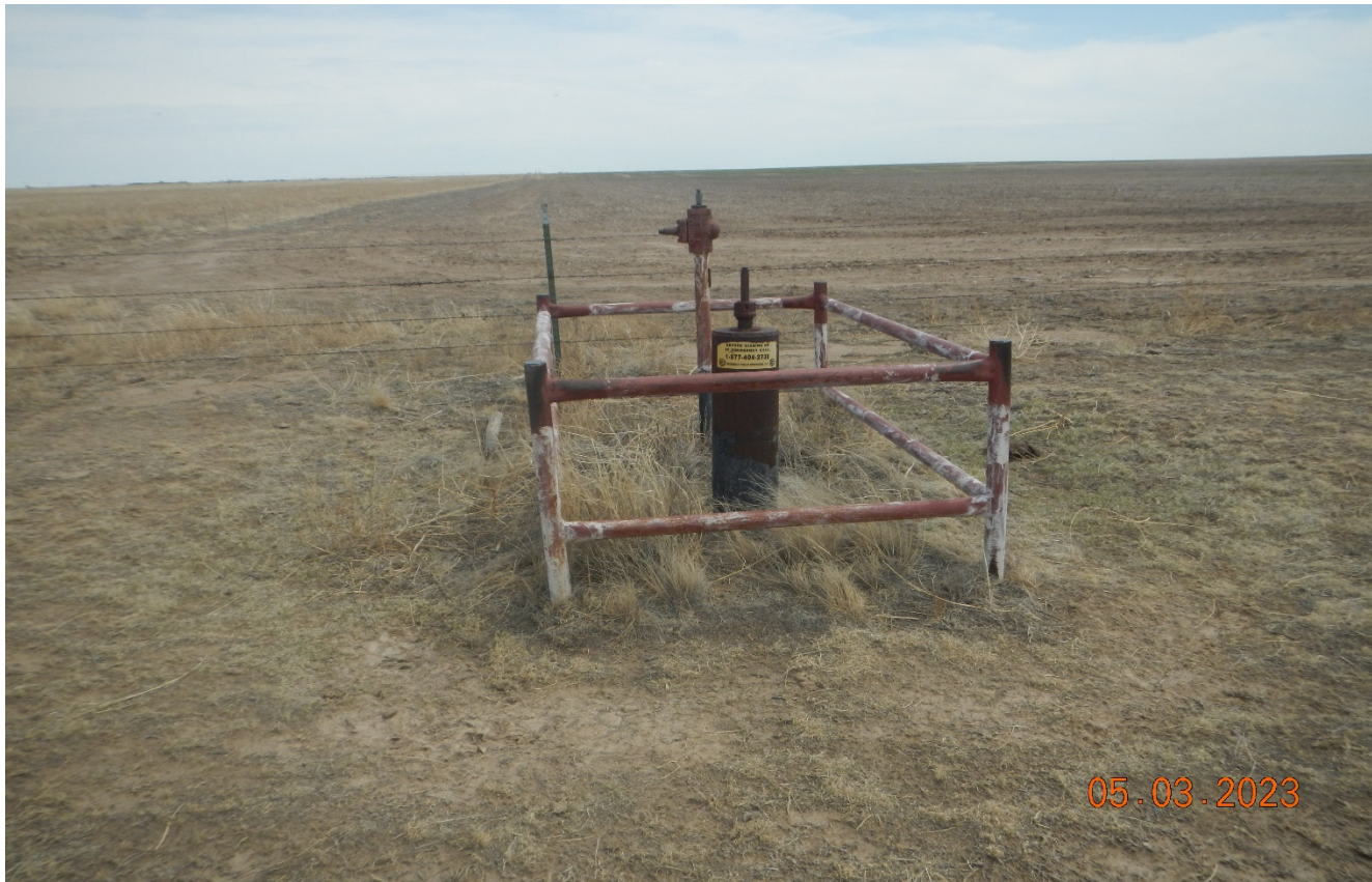
Photo 1. Approximately 100' northeast of the location is an abandoned pipeline user which must be removed.
