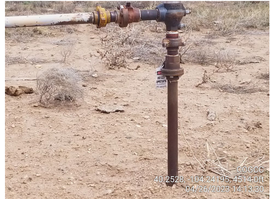
Photo 4 – Gas Meter – LOTO by Sales Operator D
