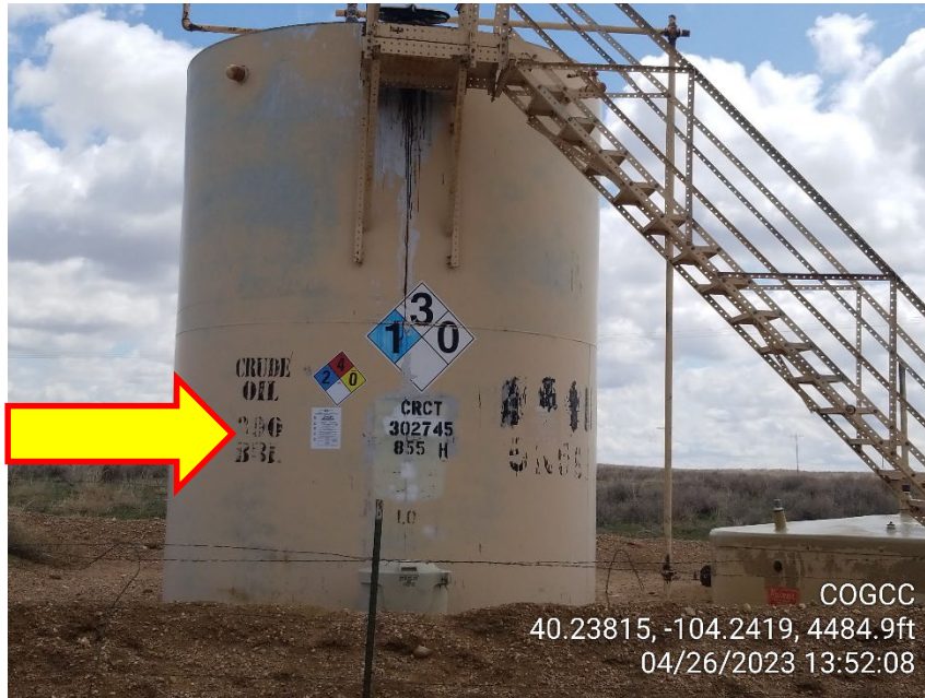
Photo 1 – Tank Battery – Capacity Label Faded
