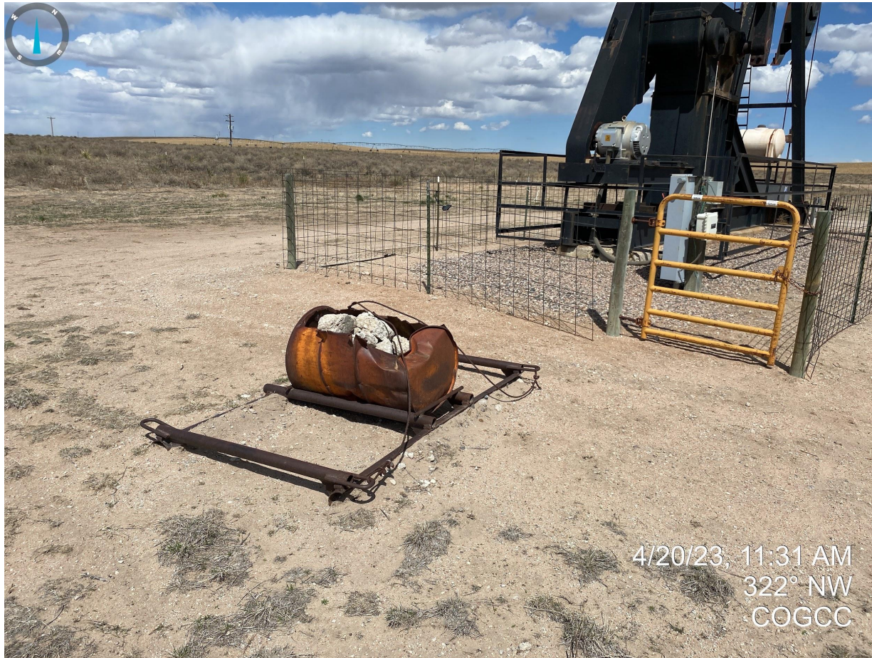
Photo 6. Road drag/maintainer being stored on location will need to be removed. Storage of equipment, supplies, etc is prohibited on location.
