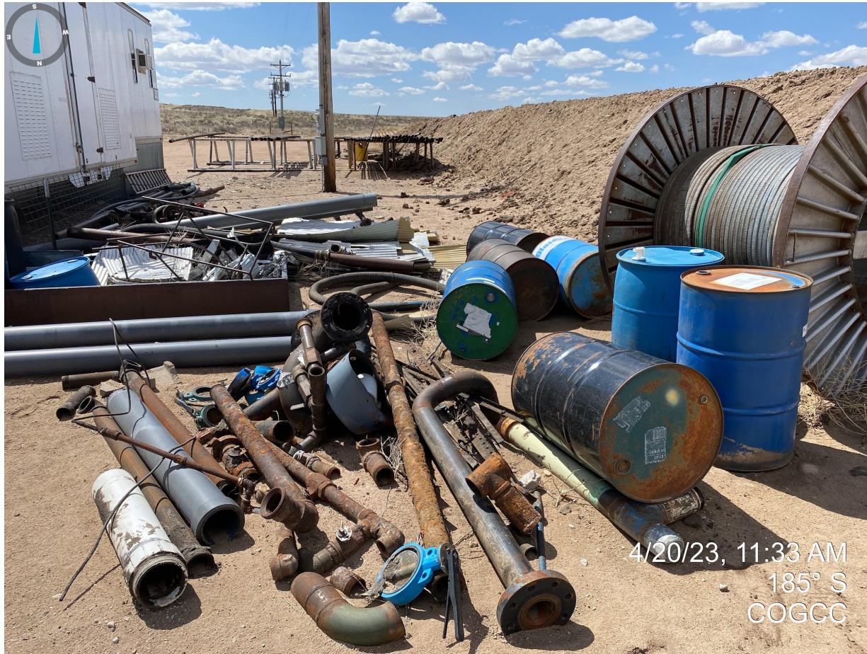
Photo 9. See comments in Photo 8. Barrels appear to be empty but are not upright or within secondary containment.
