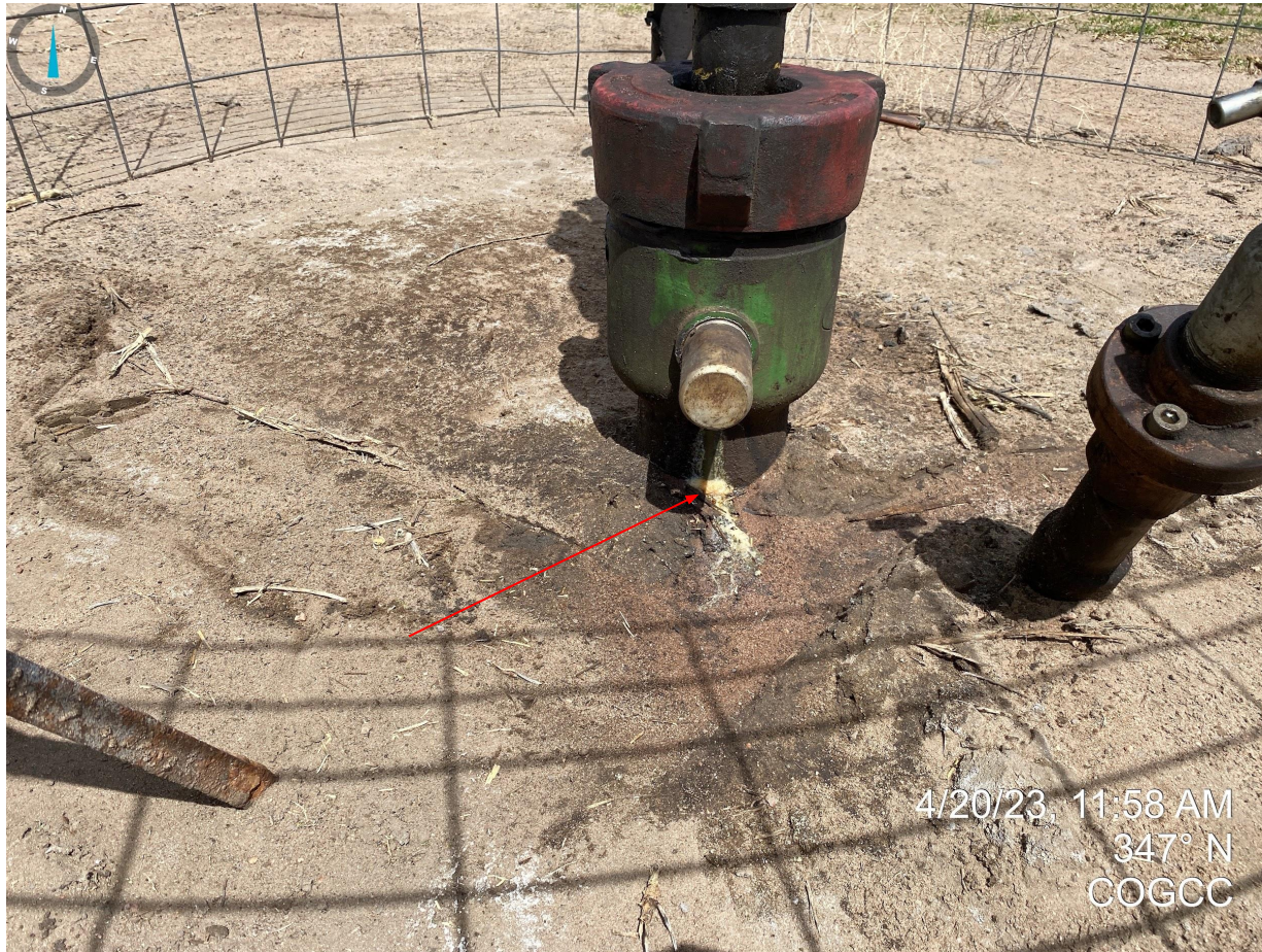
Photo 1. Stained soil will need to be properly cleaned up and disposed of per Rule 905.e. Additionally, unknown substance originating from wellhead will need to be properly disposed of and mechanical conditions will need to be inspected/maintained per Rule 608.e.
