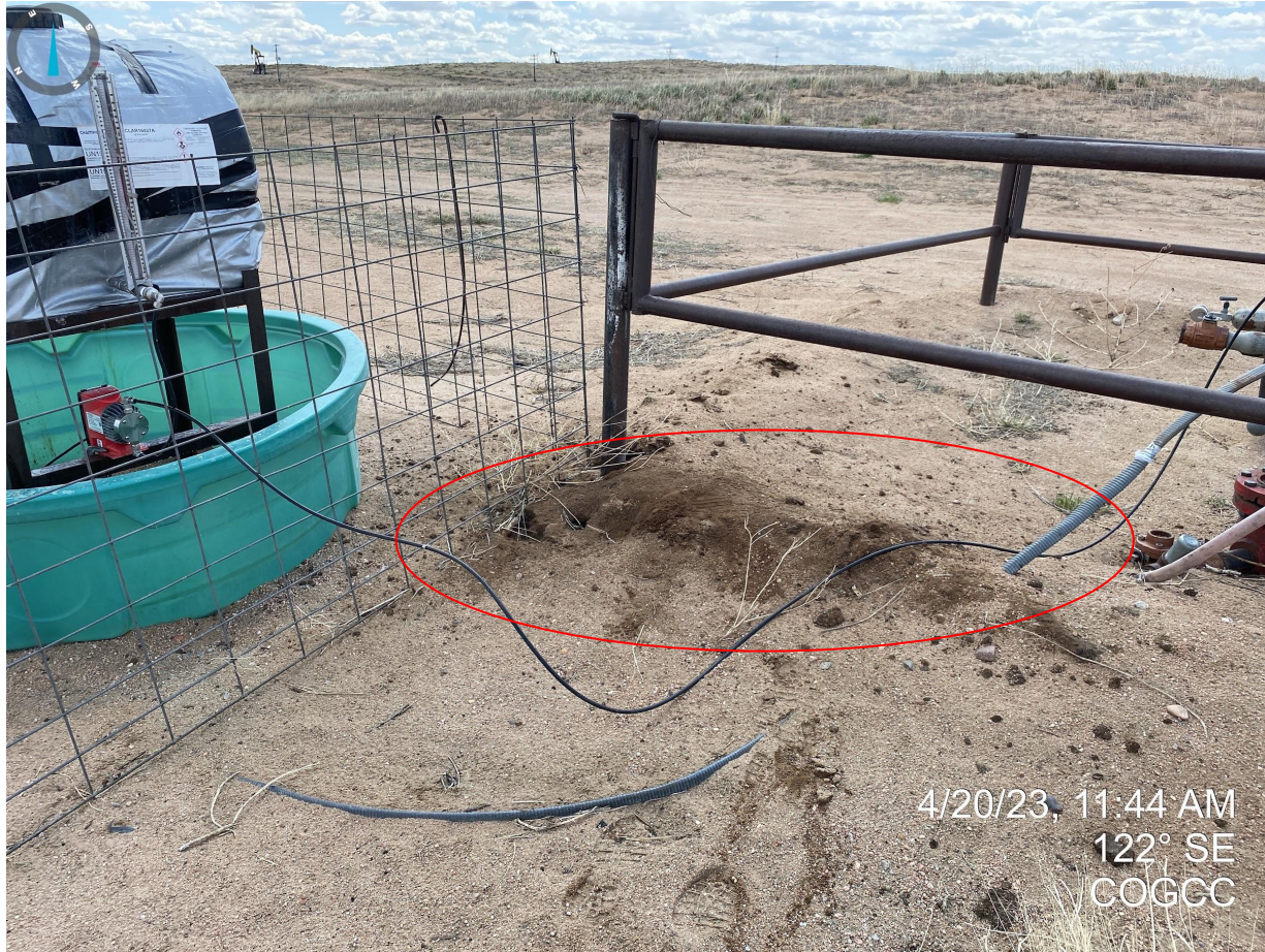
Photo 2. Stained soil near wellhead had chemical odor and will need to be properly disposed of per Rule 905.e.
