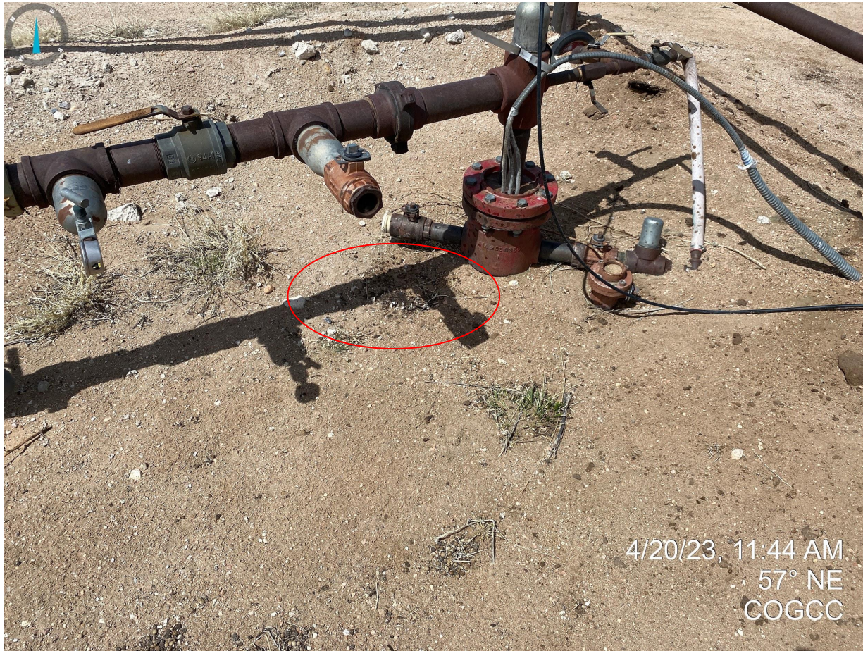
Photo 3. Stained soil at wellhead will need to be properly cleaned up per Rule 905.e.
