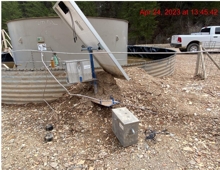
Transportation of Sediment onto Location/Encroachment on Equipment – Photo #02515
