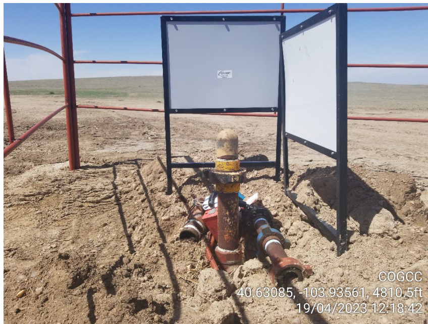
Photo 7 – Night Cap – Well appears to have been Plugged and Abandoned
