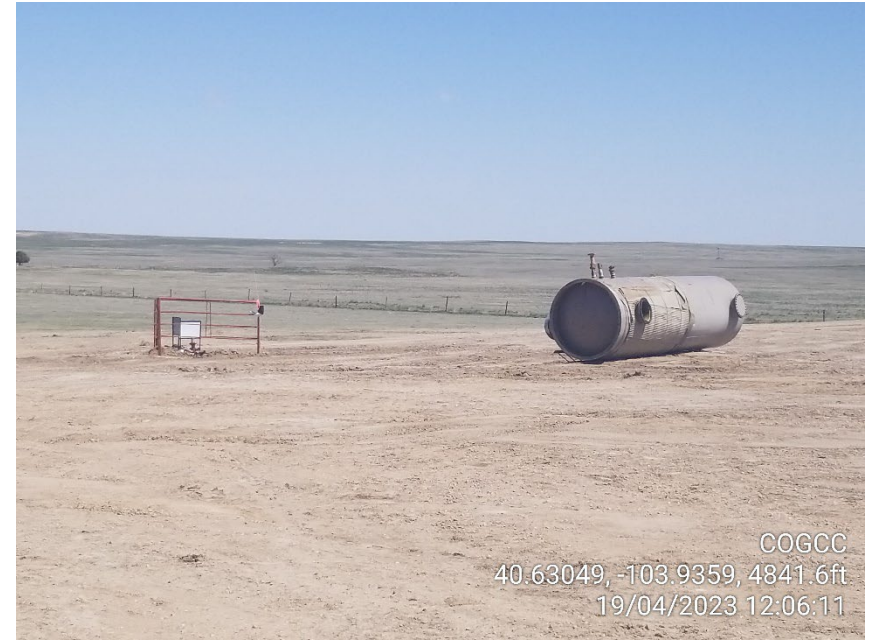
Photo 2 – Heater Treater and Wellhead
