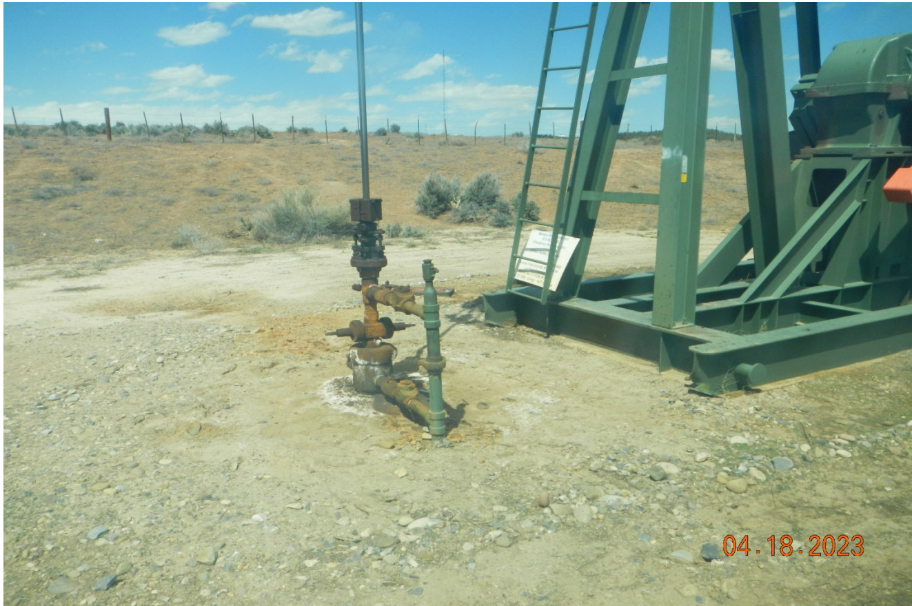
Photo 2. There is impacted soil at the wellhead that needs to be cleaned up. This issue previously cited and has not been cleaned up.
