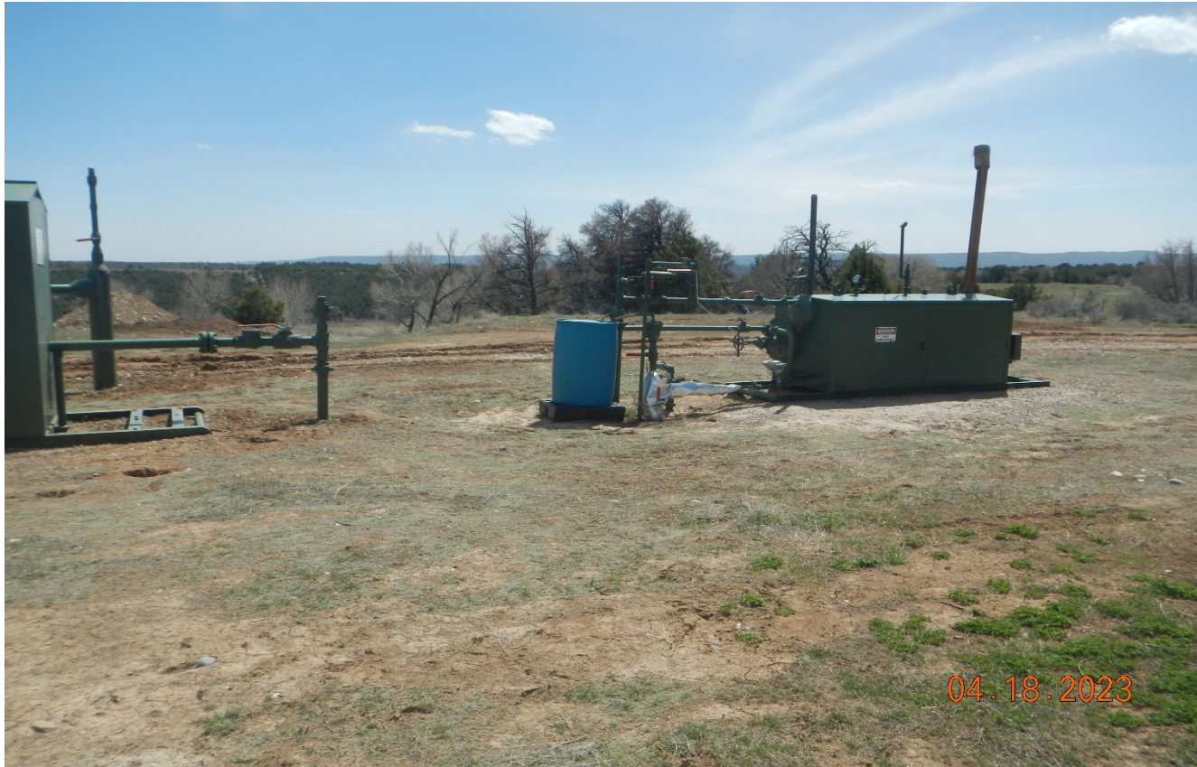
Photo 4. There is no labeling on the blue chemical drum which was previously cited.
