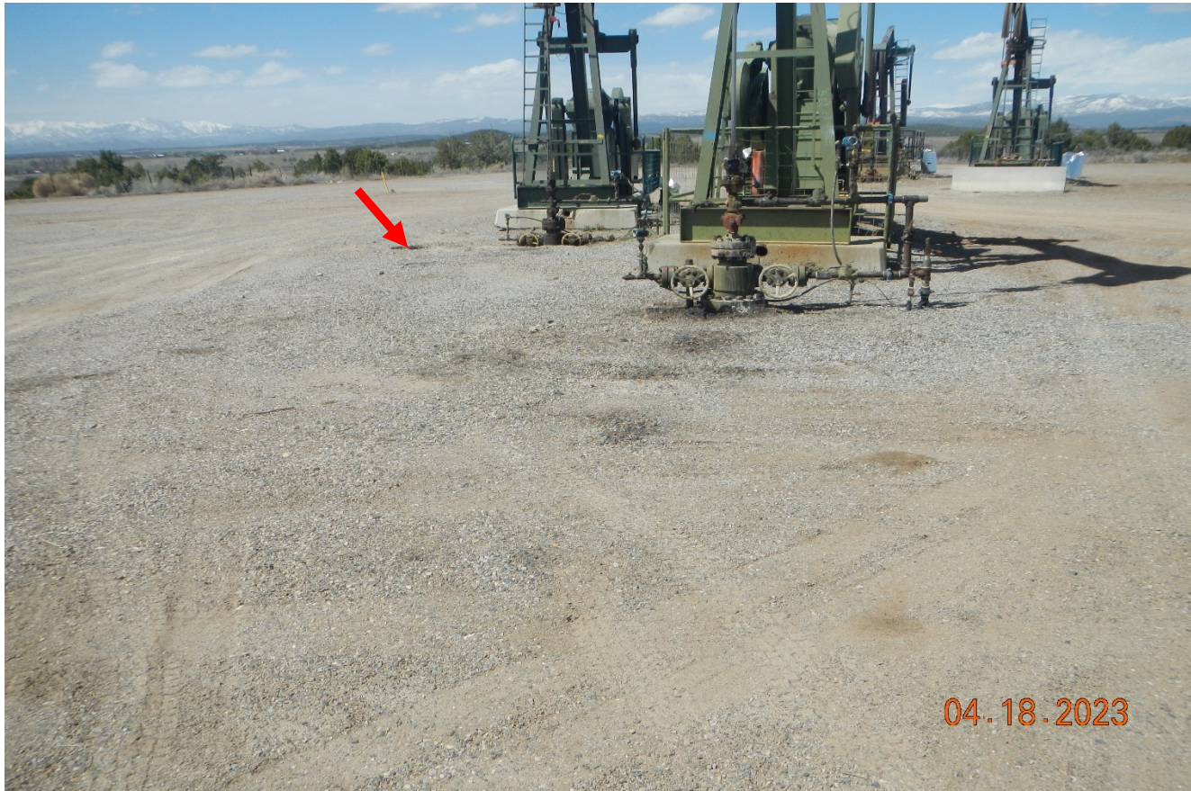
Photo 1. Facing northwest toward the wellsite. There is an open hole next to the second well at red arrow.
