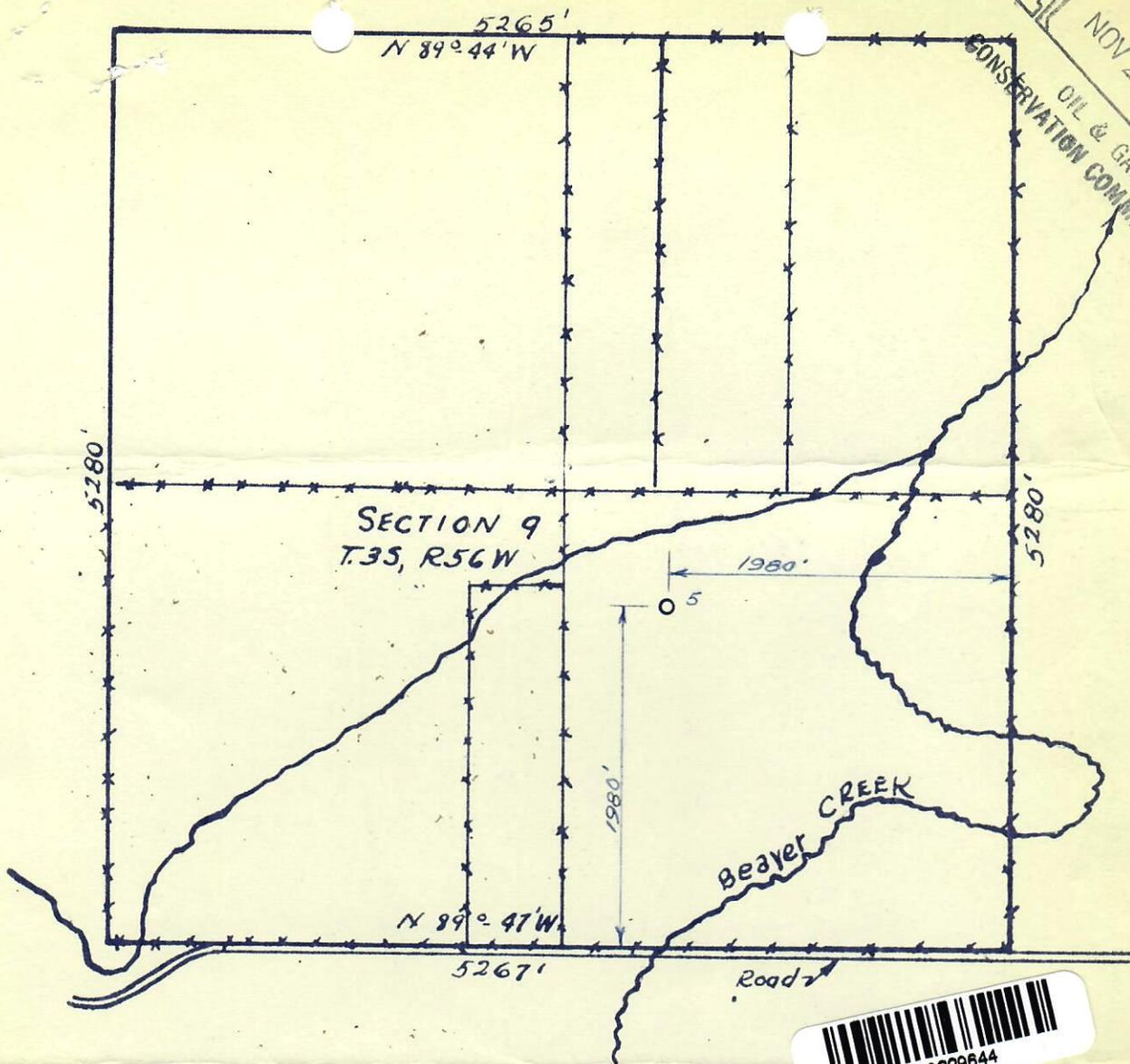
This is to certify that the above plat shows the true location of Continental Oil Company's Pierce No. 5 oil well located in Washington County, Colorado. The ground elevation of this oil well is 4664'. The above plat is from a survey dated 9-21-54.
