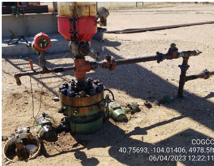
Photo 9 – Wellhead – Leaking – Stained Soil – Oil Waste
