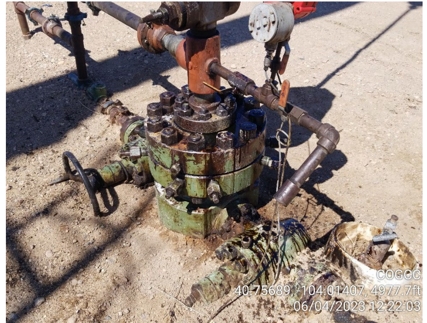
Photo 8 – Wellhead – Leaking – Stained Soil – Oil Waste
