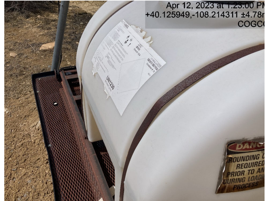
Labeling is faded and illegible
