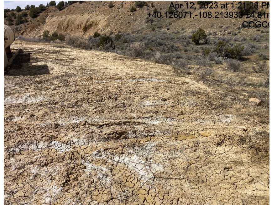
Lack of BMP's to prevent sediment migration with signs of erosion from location
