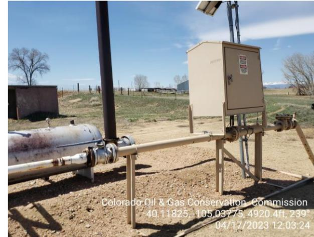
**Photo 5 Horizontal Heated Separator.**
