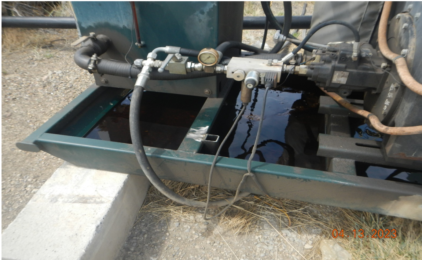
Photo 3. There is oily fluid in the engine skid that needs to be cleaned up.
