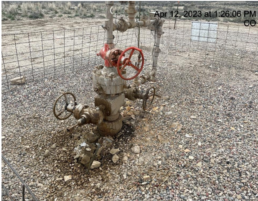
Photo # 5246 Stained soils & gravel around wellhead
