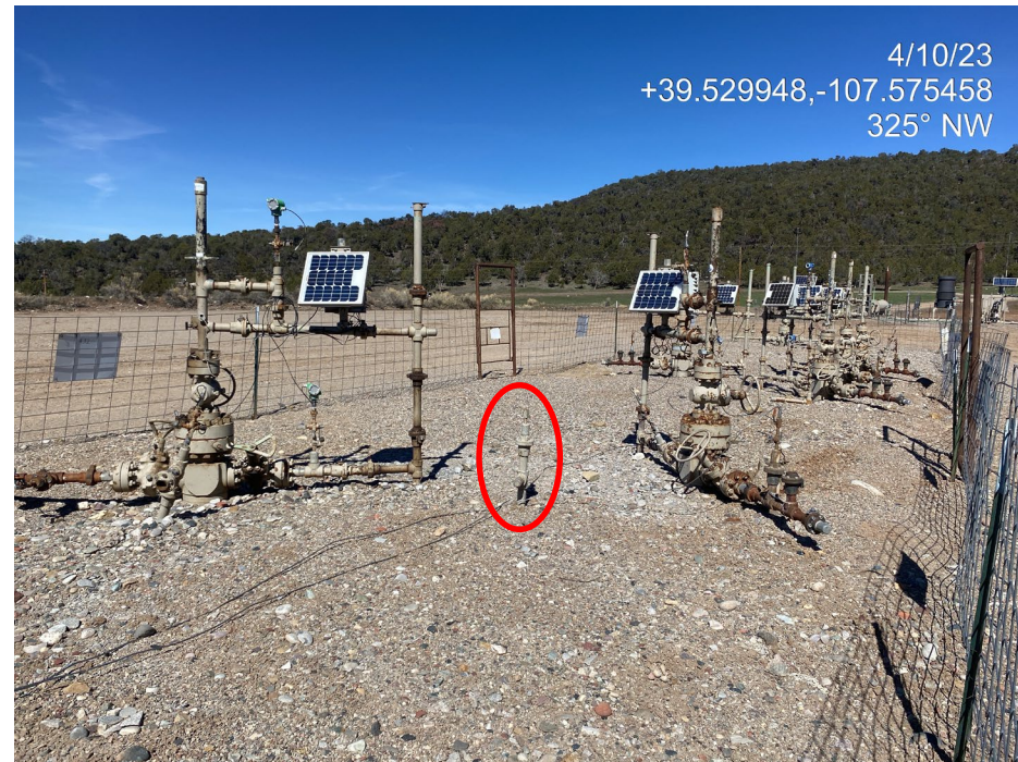
Photo 2. Photos show a flowline riser remaining at plugged and abandoned well 045-17894. OOSLAT not applied.
