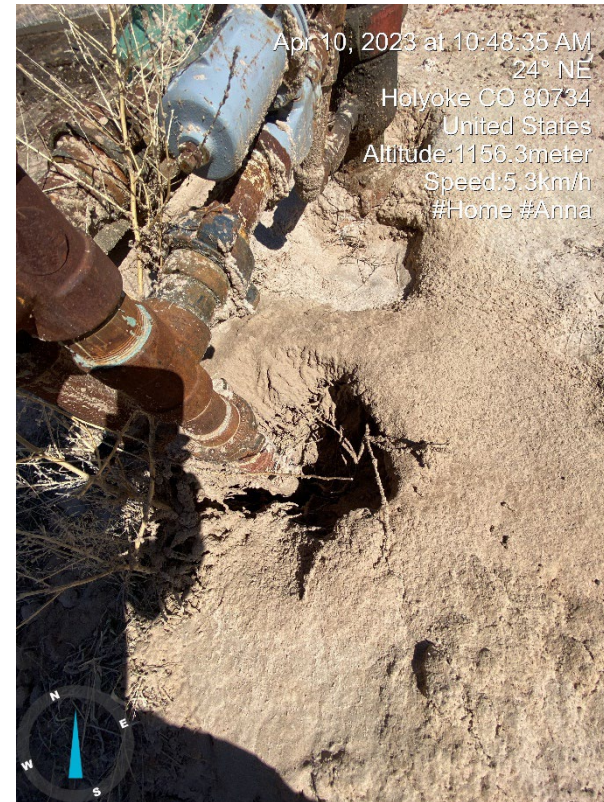
6. Gas leak on flowline blowing out of ground by wellhead.
