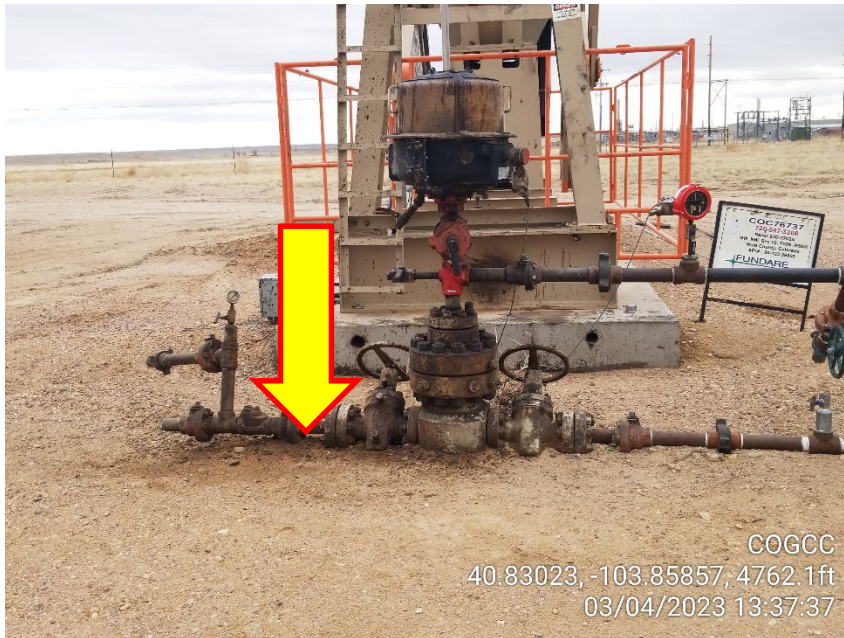
Photo 9 – 2207A Wellhead – Stained Soil
