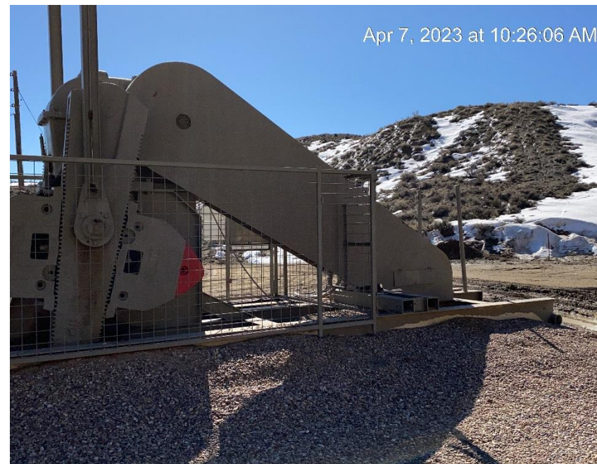
Belt guard picked up and reinstalled
