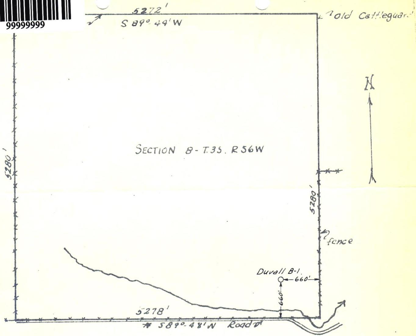
This is to certify that the above plat shows the true location of Continental Oil Company's Duvall No. B-1 oil well located in Washington County, Colorado. The ground elevation of this oil well is 4707'. The above plat is from a survey dated 9-21-54.
