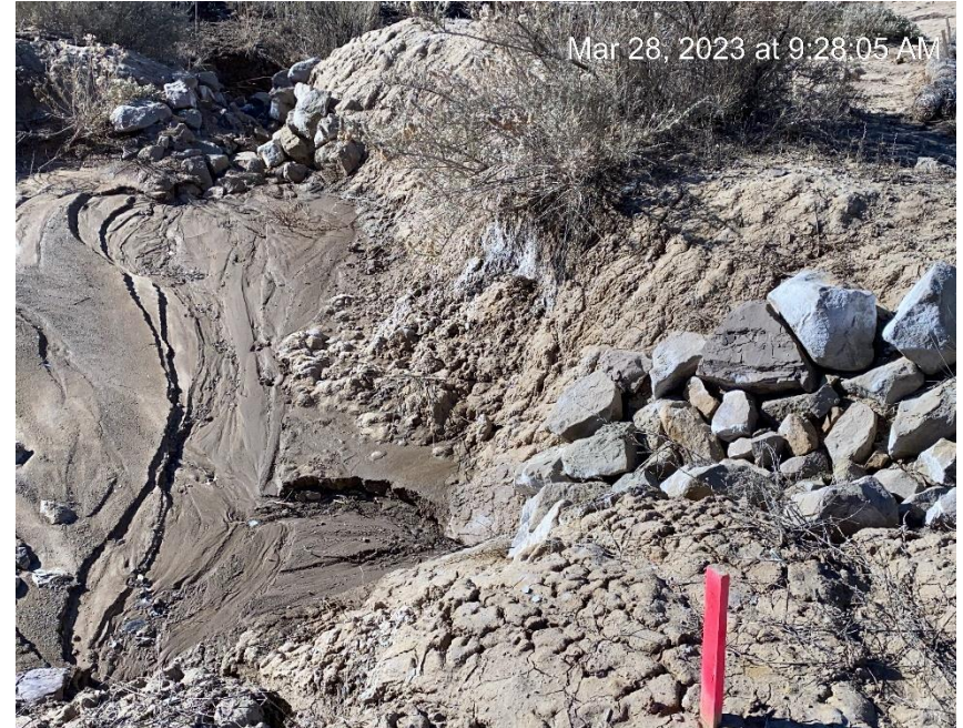
SouthEast corner trap erosion and sediment fill
