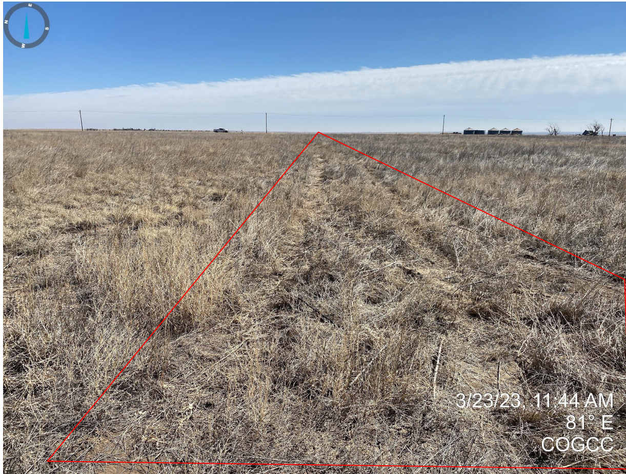
Photo 4. Facing east; the access road has not been reclaimed with evidence of road base/gravel throughout the two track road and near the former well location. Undesirable vegetation (e.g. kochia) was also observed during this inspection.
