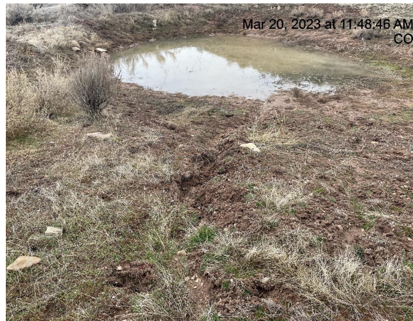
Photo # 2640 Rill erosion near settling pond NW corner
